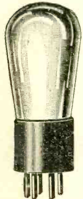
Special 201A with UX base. Note the five prongs.
